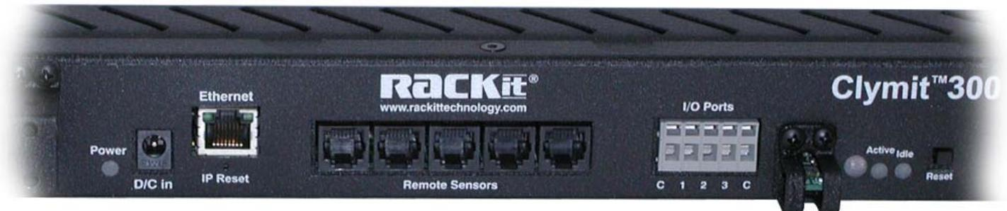
Three analog inputs are provided, numbered "1", "2", and "3"; the two terminals labeled "C" are the electrical "common", or ground. (Two "C" connections are provided for convenience; internally, they are tied together, so it doesn't matter which sensor(s) are connected to which terminal.)
