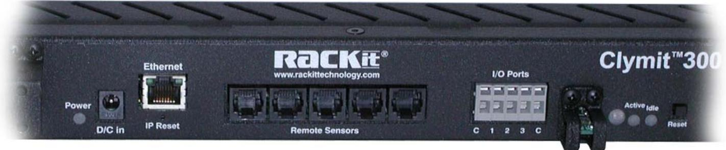
To perform a "**simple**" reset, use a paperclip or jeweler's screwdriver (using pens or pencils is not recommended, since ink or graphite particles could rub off and get into the unit) to press and hold the switch for about 15-20 seconds, or until both the IDLE and ACTIVITY LEDs light up simultaneously. Release the switch, and wait for the LEDs to resume their normal pattern (about 5 seconds) to indicate that the reset process is complete.
